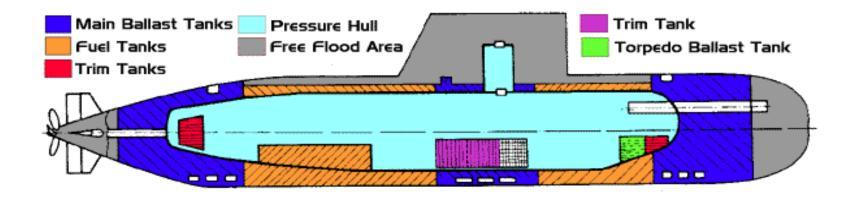
Submarines use both static and dynamic depth control. Static control uses ballast tanks between the pressure hull and the outer hull. Dynamic control uses the bow and stern planes to generate trim forces.
