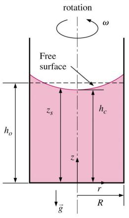
Container is rotating about the z-axis  $a_r = -r\omega^2, a_\theta = a_z = 0$   $\frac{\partial P}{\partial r} = \rho r \omega^2, \frac{\partial P}{\partial \theta} = 0, \frac{\partial P}{\partial z} = -\rho g$ Total differential of P  $dP = \rho r \omega^2 dr - \rho g dz$
