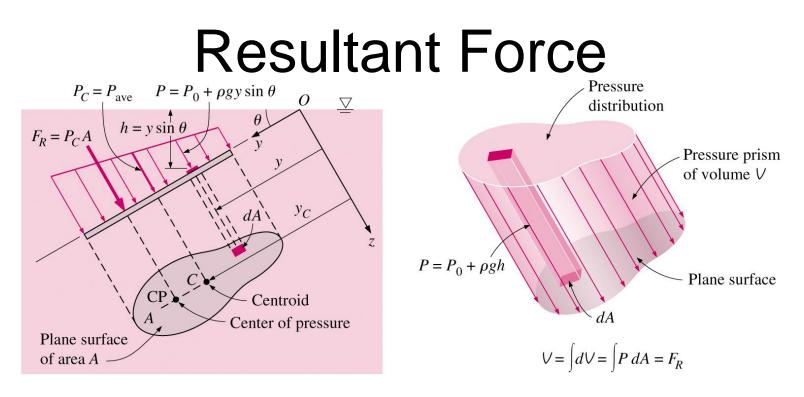
The magnitude of  $F_R$  acting on a plane surface of a completely submerged plate in a homogenous fluid is equal to the product of the pressure  $P_C$  at the centroid of the surface and the area A of the surface
