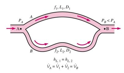
For parallel pipes, perform CV analysis between points A and B
