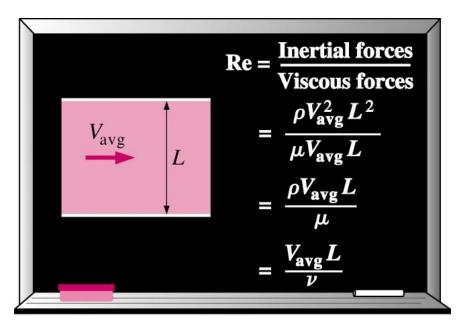
Critical Reynolds number (Re<sub>cr</sub>) for flow in a round pipe
